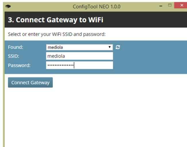
The gateway now will try to connect to your home WLAN/ Wifi. During this process the LED flashes orange until the gateway has connected to the WLAN/ Wifi successfully.
