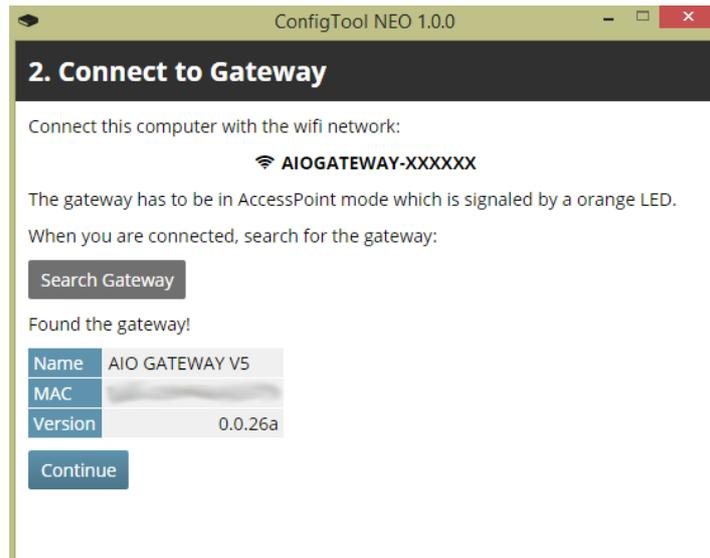
If your gateway has been detected, a confirmation will be displayed, containing the name of the device, the mac address and the current firmware version. Click on "Continue".
