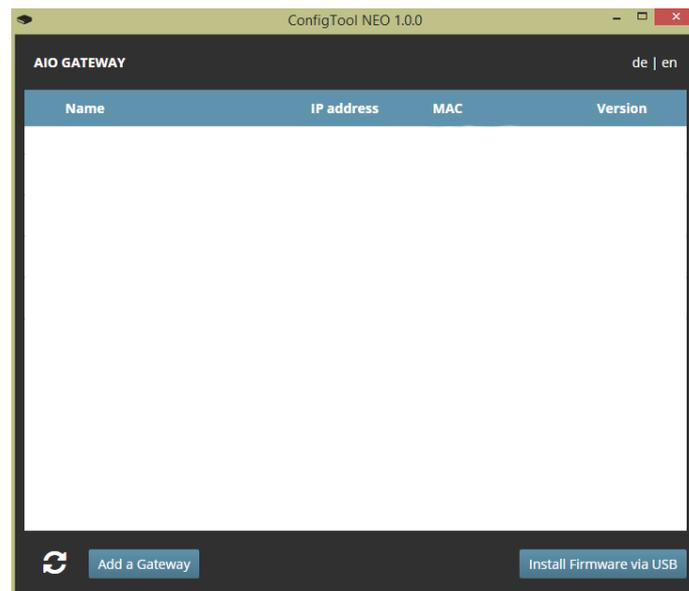
To initially configure a new AIO GATEWAY V5 with the ConfigTool NEO click on the button "Add a Gateway" on the start screen.
