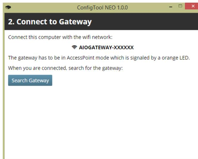
The RGB LED of the gateway should light in solid orange (access point mode). Now you can connect your computer to the gateway's own WLAN/ Wifi (not your home WLAN). For this purpose go to the WLAN/ Wifi settings of your computer and select the network named „AIOGATEWAY–XXXXXX“ (instead of XXXXXX you will see the last digits of the mac address of your gateway). Once your computer has been connected to this WLAN/ WiFi, click on "Search Gateway".
