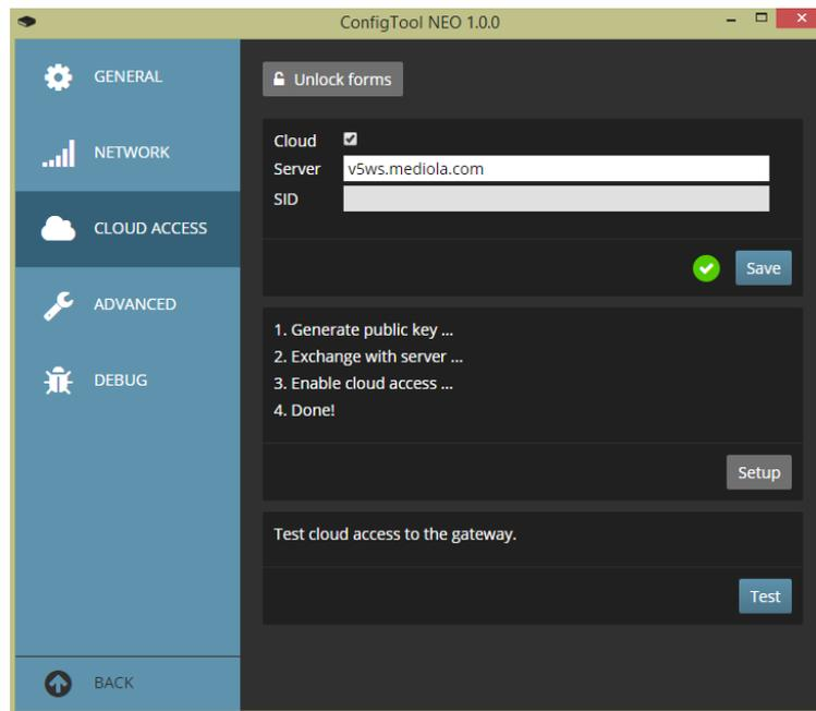
Check the mark to activate the cloud access and click "Save" (Important: Don't change the server settings) Finally click on "Setup". Now the cloud access will be activated.
